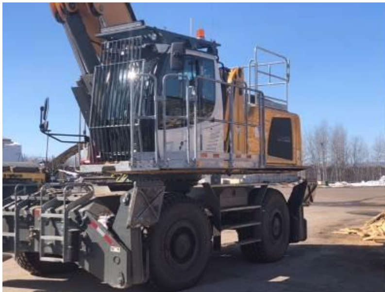
Picture #7: Example of fall-protection devices
