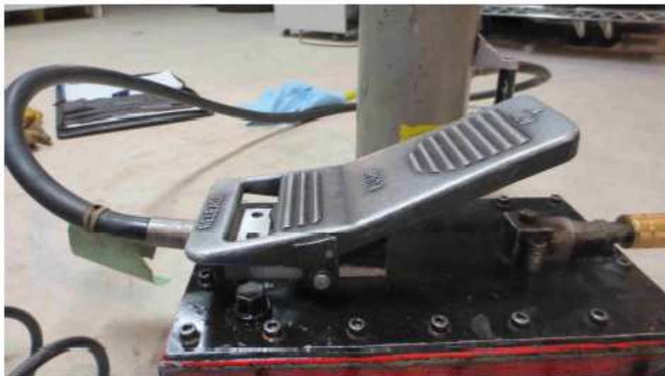
Picture #8 - Pump pedal stuck in the “Return” position
